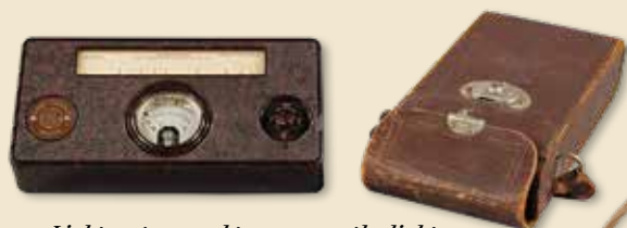
Light meter, used to measure the light intensity at which different species of birds first began singing at dawn
