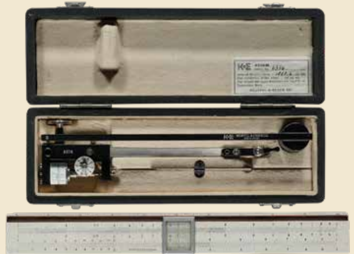
Slide rule and planimeter, used to measure distances and land areas on maps
