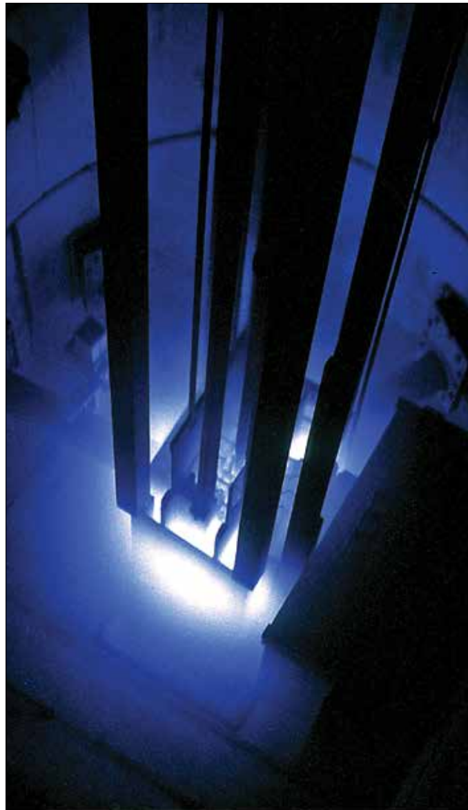
Radiation glows blue in the UW nuclear reactor. Students in NEEP 234 learn to operate the one-megawatt training reactor.
