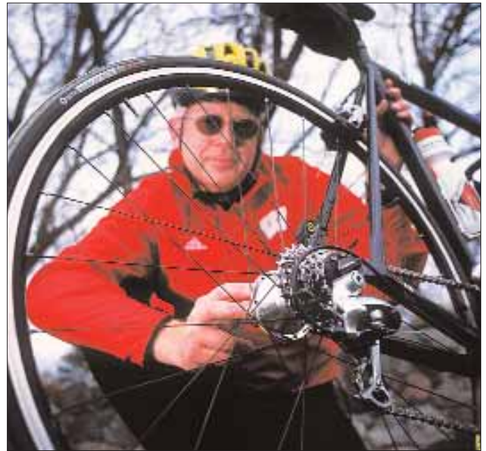
A device installed on the wheel of Jeff Sledge's bicycle logs data about the bike and its rider, including the torque and energy produced by the bike. After putting in hundreds of miles testing this "rolling laboratory," Sledge will soon learn how the equipment does in cycling's premier event, the Tour de France.
