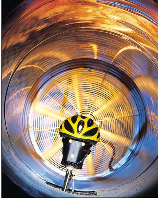
One tester decided to find out if all those vents in newfangled bike helmets are just a gimmick. So he built a wind tunnel, and he discovered that the extra vents do indeed help bikers to keep a cool head — without compromising safety.
